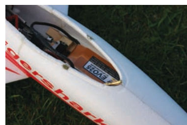
Above: Peering into the fuselage you can just see the adjusters for the two elevators
